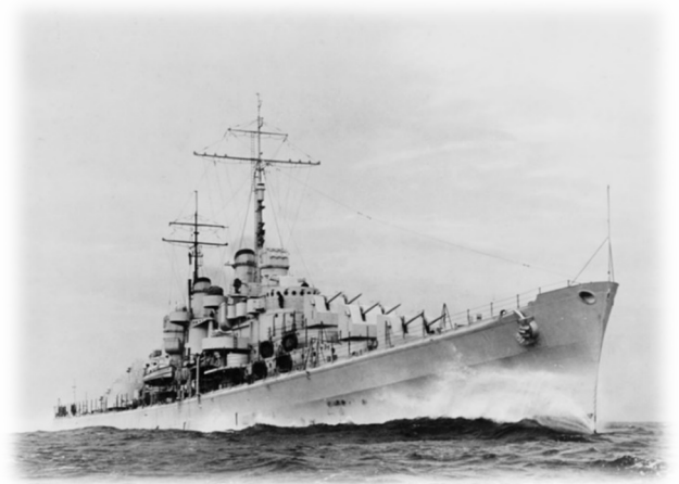
Above: The Atlanta class was a light anti-aircraft cruiser with 8 double 5" / 38 dual purpose guns as well as dozens of lighter anti-aircraft cannons. Radar assisted gunnery made these ships especially deadly to Japanese aircraft.
